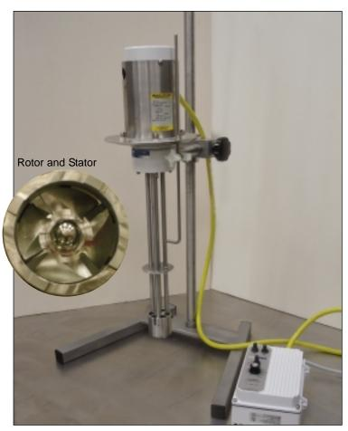
The Model CJ-4E Reversible Homogenizing Mixer was specifically designed for batch sizes from 1 to 5 gallons. With a 1.8" diameter 10,000 RPM axial flow rotor, high shear rates approaching 50,000 reciprocal seconds are obtained. These high shear rates are capable of de-agglomerating powders in liquids and emulsifying difficult immiscible liquid mixtures.
