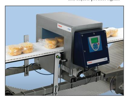
on the fly to assure highperformance and to eliminate false rejects. The result is up to 50% smaller diameter metal can be detected in many previously difficult metal detection applications.
